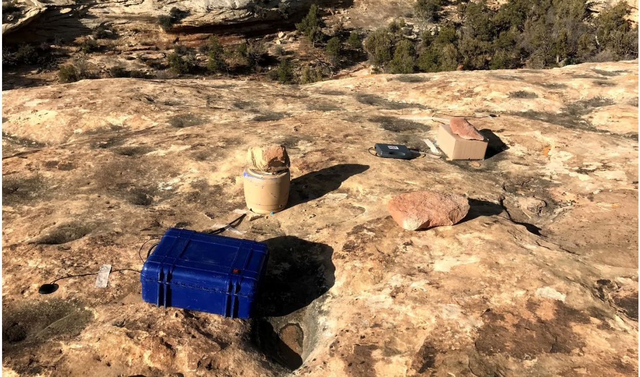
Figure 1. Deployed instruments covered using a box and a bucket to minimize noise from wind and rain. Trillium Compact digitizer and accessories are located in the blue case, while the Raspberry Shake is powered by a small battery in the gray case.
